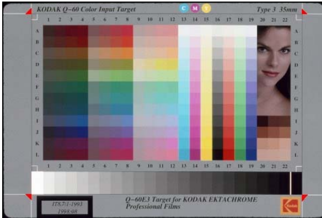
Q60 Target combines both the Grey-scale and Color targets. This target is standardized by American National Standard IT8.7/1.
